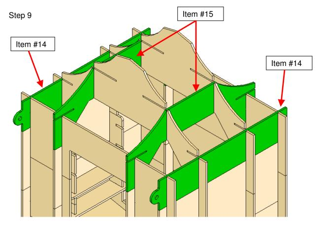
Install the 5 foot Wall Top pieces with the Rod Holes towards the Front Install the 5 foot rafters
