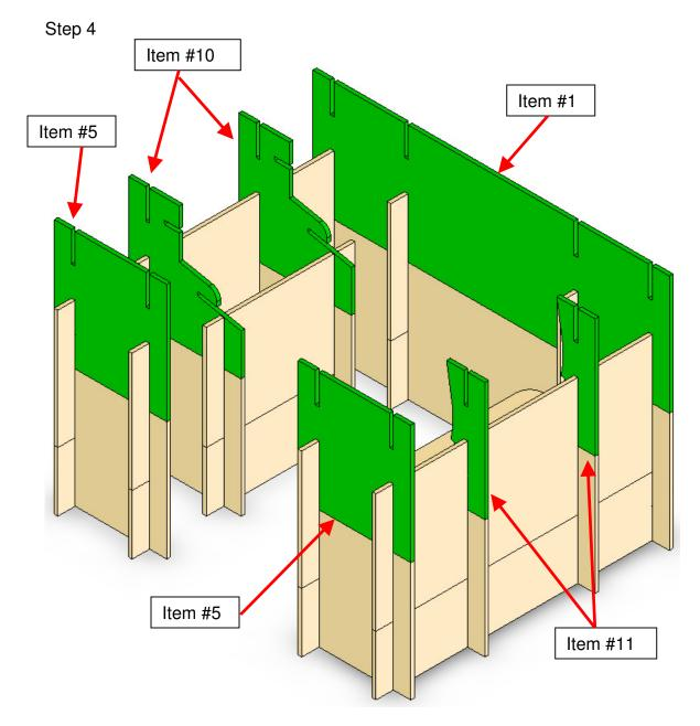
Install the next level 22.75 inch Front walls and 6 foot Back wall pieces, plus the Seat Back parts on the Bench Side and the Stand Supports on the Stand Side
