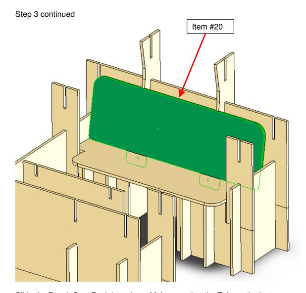
Slide the Bench Seat Back into place. Make sure that the Tabs at the bottom slide into the Bench Seat and into the supports below.
