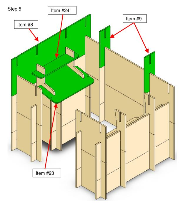
Install the 5 foot Side Wall and the H pieces for the Back wall. Slide the Desk Top into place and set in the first Shelf.
