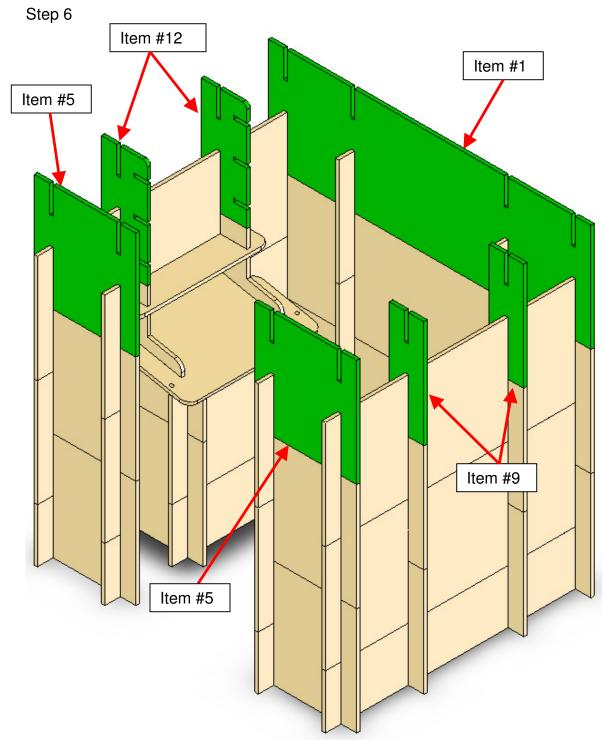
Install the next level 22.75 inch Front and 6 foot Back Wall pieces plus the next level Shelf Supports and H Pieces in the Side Walls
