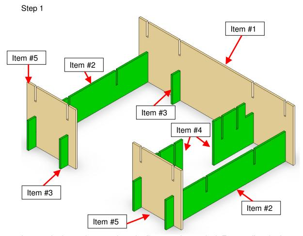
Lay out the base pieces and set the first row of 22.75 inch Front wall and 6 foot Back Wall pieces
