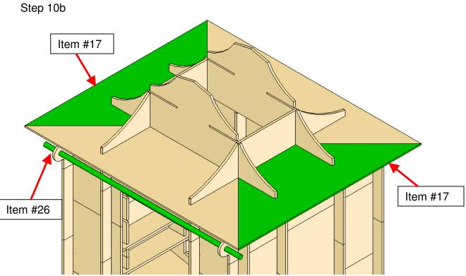
Slide in the Medium angled roof pieces from the sides. Insert the Curtain Rod (with curtain - not shown)
