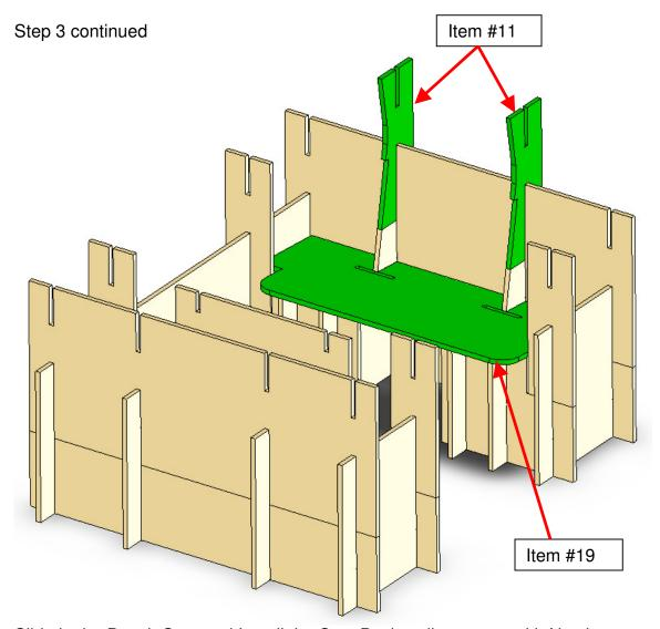
Slide in the Bench Seat and Install the Seat Back wall supports with Notches as shown
