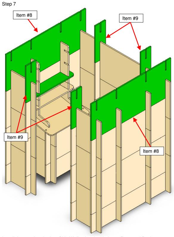
Install the next level 5 foot Side Walls plus the H pieces Front and Back. Add in additional Shelf as desired
